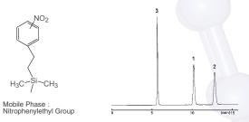
4.6mml.D. x 250mm Column size Mobile phase Toluene/ Hexane = 25/75 Flow rate 1.0ml/min 30oC Temperature Detection UV 325nm
